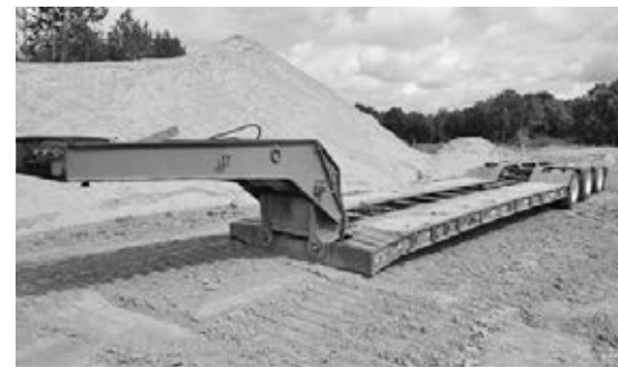
'91 Talbert 50-ton lowboy, NGB, hyd., detach, air ride, 102" wide, tires 255/70R22.5, good cond. for age, $23,900 or best offer.
