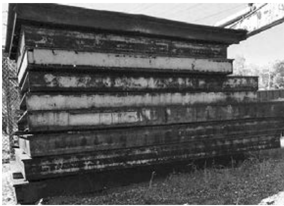
Deck plate w/8" H-beams on frame, (1) 10'10"x9'11"x8" frame, (3) 11'2"x11'x8" frames, (2) 11'9"x7'5"x8" frames, (1) 8'4"x9'11"x8" frame, (1) 8'x9'11"x8" frame, all check plates are approx. 7/8" thick, all steel beams are 8" H-beams, (412) 384-2008
