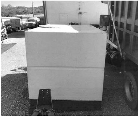
Steel fuel tank, manufactured by Highland, heavy steel tank, approx. 1/4" thick, plate 10'10" long, 6'6" wide, 6' tall, sits on (2) 12" H-beams, approx. 3100-gal., (412) 384-2008
