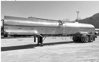
'95 Barbell, S.S. barrel, S.S. subframe, 2-compt., 6900-gal. cap., tdm. axle, alum. rims, air ride susp., $35,000.
