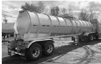
'99 Polar, alum. barrel, steel subframe, 8500-gal. cap., dbl. conical, 1-compt., tdm., pol. rims, call for a great deal!
