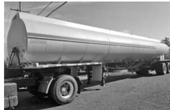
'00 Heil, alum. barrel & subframe, 9800-gal. cap., 4-compt., tdm. axle, spg. susp., $37,000.
