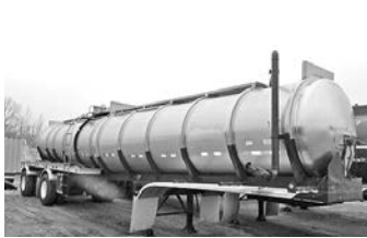
'85 Brenner, S.S. barrel, steel sub-frame, 7000-gal., dbl. conical, tdm. w/spread, pilot whls.
