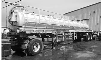
'10 Dragon , alum. barrel, stl. subframe, 6300-gal., single compt., tdm. axle, call for pricing.
