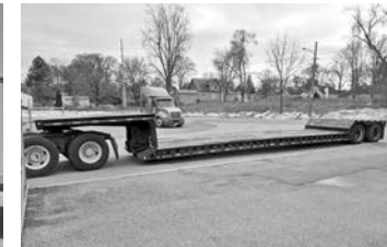
1997 Trail King 48'x102", all steel double drop, ready to go to work.
