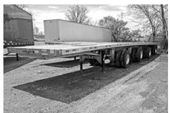
(2) 2018 Manac quad axle flats , all aluminum, Hendrickson INTRAAX air ride.
