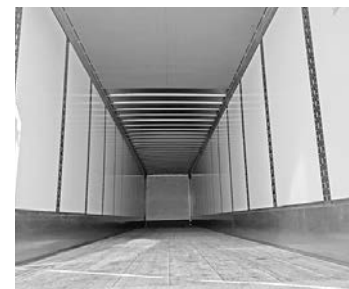
(40) 2019 Hyundai composite vans available still this year! Tire inflation, external rub rails, galvanized coupler & CMs, 24K floor .
