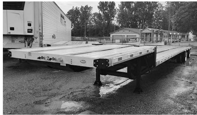
2019 Dorsey combo step decks, rear sldg. axle, chain tie-downs, 22.5 aluminum wheels.
