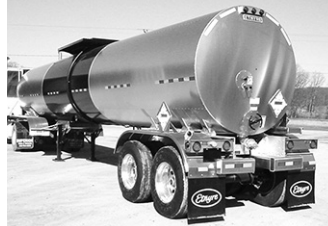
New Etnyre asphalt trlr., 7250-gal., all alum., air ride susp., 22.5 tires on alum. whls.
