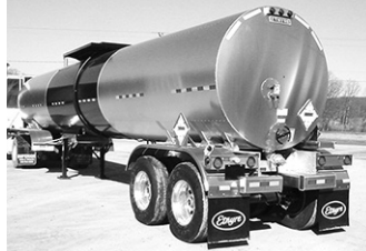
New Etnyre asphalt trlr., 7250-gal., all alum., air ride susp., 22.5 tires on alum. whls.
