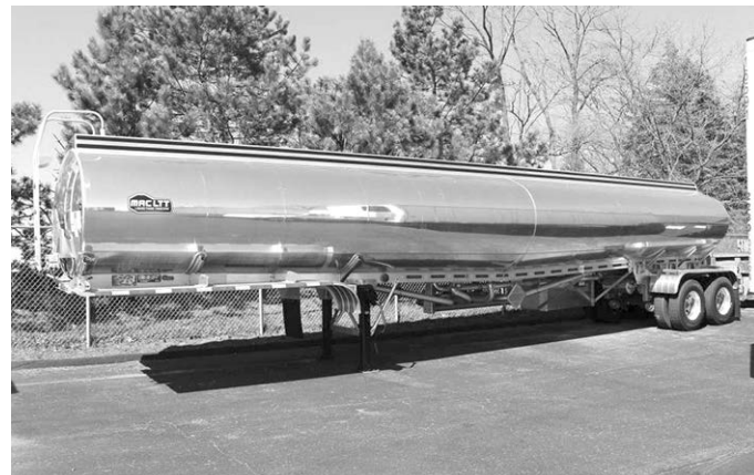
New '17 MAC LTT DOT 406, 4-compt., straight elliptical, compts. are 3500/1200/2000/2800 gal. all w/dbl. bulkheads, Hend. air ride susp., 11R22.5 tires, alum. whls., mention ad to get special online pricing of $76,500 + F.E.T., F.O.B. Dearborn, MI.
