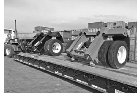
'18 Flip axle attachment, Ridewell air susp., air brakes, 25,000 cap., $13,999. F.O.B. Dearborn, MI.
