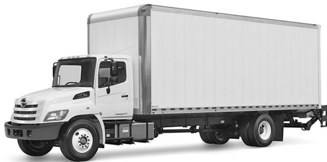
New '18 Morgan 24' or 26'x103"x102" GVSD alum. dry freight van body, full plywood lining, Hi-Lo pkg. (incl. 23" threshold plate, (4) extra CM's @ rear, reinforced frt. end & 12" scuff), translucent roof, (2) rows of E-track, 10" dock, ICC bumper. Call for lead time & details.
