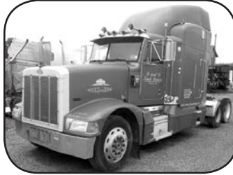
'96 Pete 377 tractor, Det. Series 60, 380/430 hp, Fuller RTLO16610B, Super 10 trans., Eaton 404 rears, 3.90 ratio, Pete air leaf susp., hub pilot whls., 252" WB.
