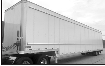
'18 Stoughton drop deck dry van, 53' w/18" drop, 126" ins. ht., plate construction, California legal, air ride, log. slots.
