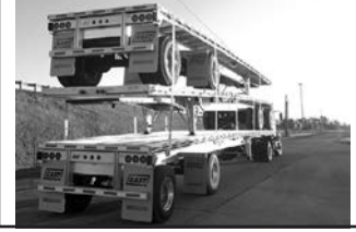
(4) '19 East 48' alum. spreads, sldg. winches, J-hooks, alum. whls., BSTN rubber, (2) 53' w/sldg. rear axle.
