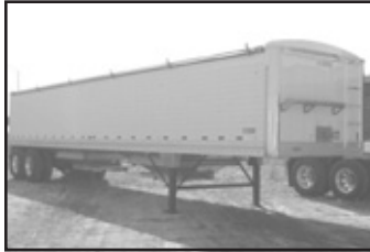
(2) '12 Stoughton alum. ag hopper, 40'x96", 68" sides, air ride susp., 29"x32" gates w/24" ground clearance, 11R22.5 tires, alum. whls., 18 oz. black Shurco ShurLok tarp.
