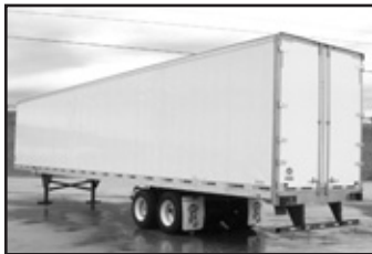
(12) '13 Utility 53' 4000 DX dry vans, 100" ins. width, air ride susp., oak floor, alum. roof, 22.5 LP tires on steel whls.
