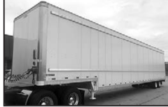
(2) '19 Stoughton Z-plate composite drop frame dry vans , auto spec w/(2) rows of plastic scuff side walls, corrugated scuff in ceiling, (2) rows of ext. rub rails, tire inflation, 125" door openings.
