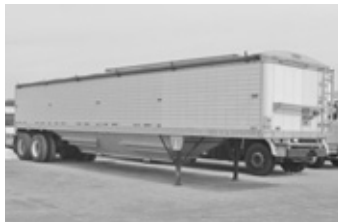
'94 Tempte 40'x56" hopper, air ride, 11x22.5 tires on steel Budds, roll tarp.
