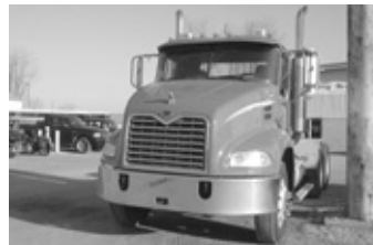
'07 Mack CXN613 day cab, 460 Mack, 13 spd., camelback susp., bronze bushings, Mack rears, 3-line wet kit, alum. rear 1/2 fenders, 3/8 heavy frame.
