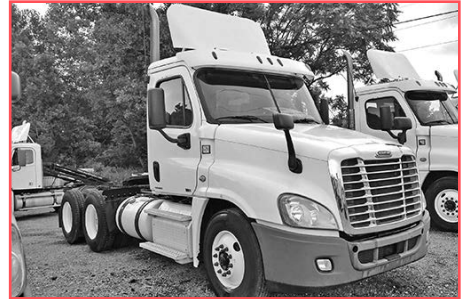
'12 FTL Cascadia 125 day cab , DD13, 435-490 hp, eng. brake, 10 spd., 3.70 ratio, air ride, 178" WB, $39,900.
