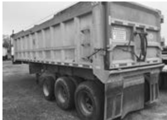
'95 MAC 32'x30" tri-axle dump, alum. frame, air ride, 11R22.5 tires on alum. whls., 2-way gate, lift axle. Also: '00 Benson 22'x66" tdm. alum. dump.
