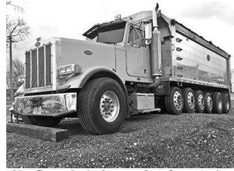
'05 Pete 359 dump, C13 Cat, 435 hp, 8LL trans., 46R, Chalmers susp., (4) lift axles, frt.-to-back tarp, all alum. whls.
