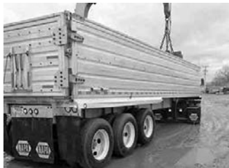
'16 Dragon 36' tri-axle dump, alum. frame, 60" sides, air ride, full steel liner, 11R24.5 tires on alum. whls.
