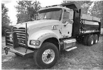
'11 Mack Granite, MP8, 445 hp, 310M trans., 18F, 46R, camelback susp., new Beaucroc 18' Hardox steel bed.
