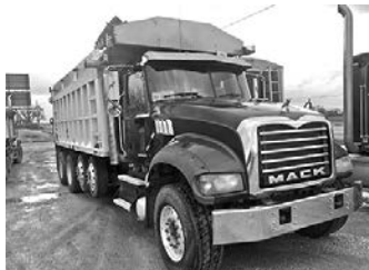
'09 Mack GU713, 445 hp, 13 spd. Mack, 44R, camelback susp., 18' alum. bed, frt.-to-back tarp.
