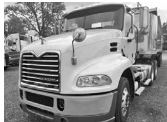
'14 Mack CXN613, MP8, 445 hp, M-Drive, 40R, air ride. Also: '13 w/ same specs.
