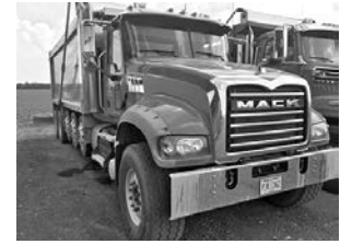
'16 Mack GU713, MP8, 445 eng., 310M trans., 44R, camelback susp., 20' Alfab alum. bed.
