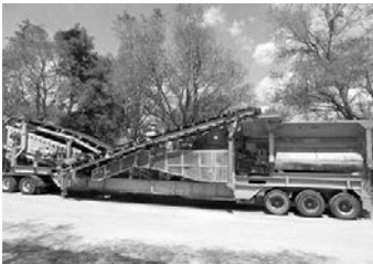
Eagle Crusher 1200 closed circuit impactor plant, twin deck screen box, 2.5" screen & 1" screen, return conveyor, magnet, vibrating feeder, Cat 3406. . . . Call
