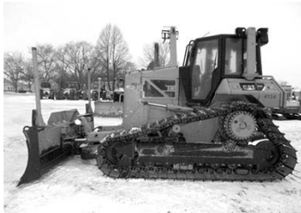
'07 Cat D6N LGP dozer, 6-way, A/C cab, diff. steer, plumbed for GPS, System One U/C, plumbed for ripper, U/C is around 80%. . . . . $64,500
