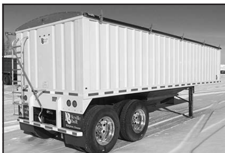
'18 Neville steel hopper trlr., brand NEW, just arrived, 28', alum. O.S. whls., Shurco roll tarp, vertical rib sides, spg. susp. . . Call
