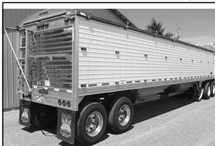
'16 Timpte, 40'x96"x72", (2) ag hoppers, 11R22.5, alum. whls., roll tarp, air ride, S.S. rear, (2) rows of (9) LED lights per side. . . . . $35,900
