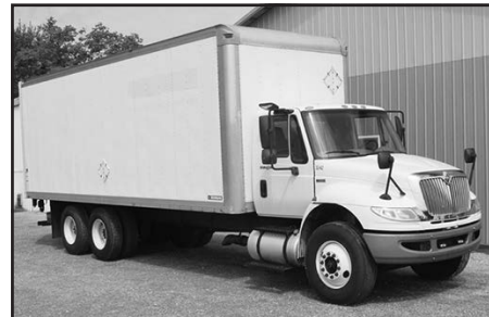
'12 Int'l. 4400, IDEALEASE, 233,000 miles, DT466, 300 hp, 10 spd., 4.88 ratio, air ride, Morgan 26'x102"x103" van, w/4000 lb. platform liftgate, nice. . . . . $36,900
