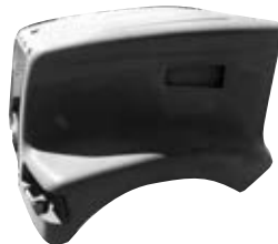
Volvo VHD set forward axle hood shell.
