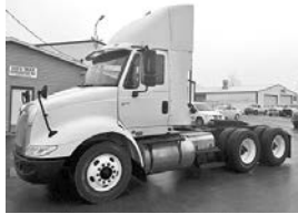
'07 Int'l., ISM Cum., 370 hp, Allison 4000HS auto. trans., air ride, air shield can be removed, $33,900.
