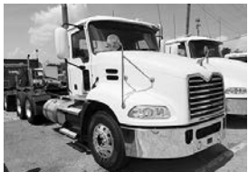
'12 Mack CXU613 , day cab, 445C MP8 Mack, 10 spd. Fuller FRO18210C, Jake, air ride, single frame, wood look dash, pwr. locks, A/C, cruise, 3.90 ratio, fully serviced & D.O.T. ready, PS, tilt, alum. rims.
