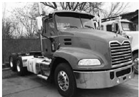
New '16 Mack Pinnacle CXU613 , MP8-505 Mack eng, 505 hp, dsl., 13 spd. O.D., eng. brake, air ride susp., 3.90 ratio, 11R22.5 tires, all alum. whls., 185" WB, tdm., 12F, 40R, call.
